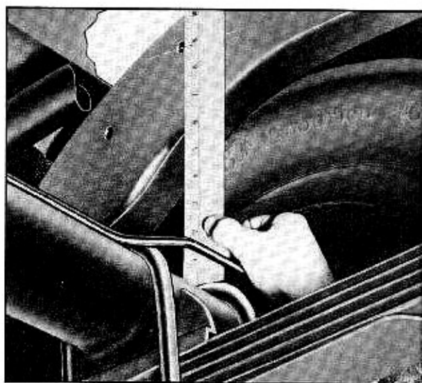
Fig. 6-5 Measuring Rear Spring Height
